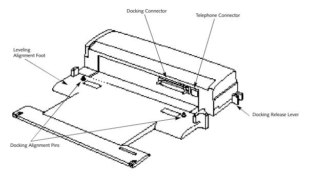
Figure 4-19 Port Replicator Front View
